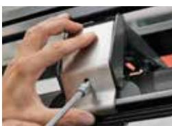
7) After you have positioned the roof rack on the roof, slide legs for symmetrical alignment heightwise and depthwise.
