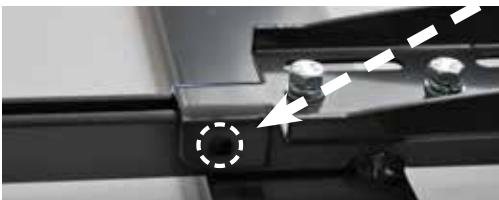
4) For extreme off-road use, it is also possible to lock the leg further by a through bolt by drilling a hole in the crosspiece (marked by an arrow in the picture). This operation should be carried out only after the roof rack has been mounted and aligned to the roof.
