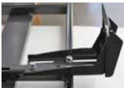
3B) Insert just one rectangular bolt in the crosspiece; the other two should go into the slot of the outer frame. Attach the leg by the proper bolts without tightening. All nuts and bolts should be permanently tightened only after the roof rack has been mounted and aligned.
