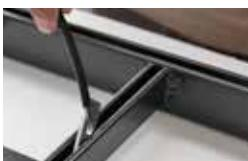
5) In order to remove rectangular nuts from the various slots, a proper magnet is provided which will facilitate this operation.
